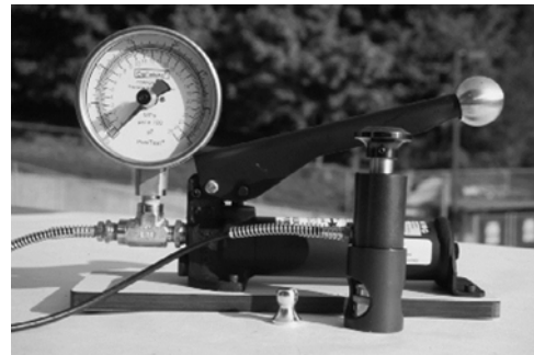
Figure 38. Tensile adhesion test kit.
