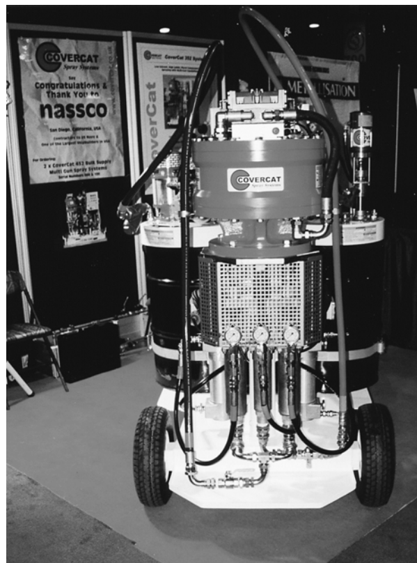
Figure 4. Plural-component proportioning system.
