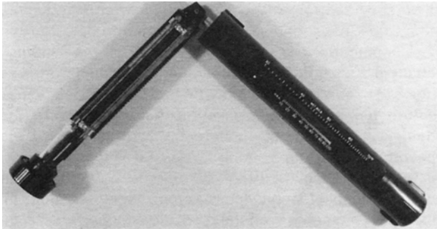
Figure 1. Sling psychrometer used for measuring wet and dry bulb temperatures in order to establish relative humidity and dew point. The instrument is spun in the air to reach temperature stabilization.
