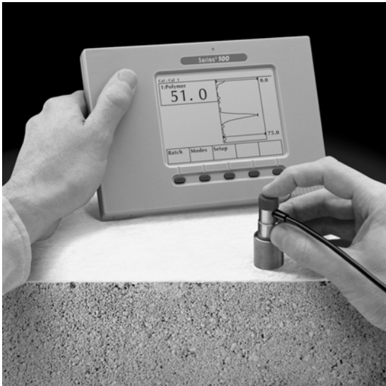
Figure 27. PosiTest 100 ultrasonic gauge.
