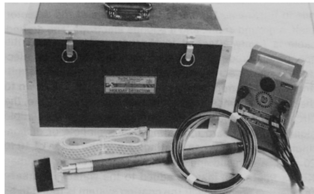
Figure 37. D.E. Stearns high-voltage holiday detector used for non-conductive coatings applied to conductive substrates.
