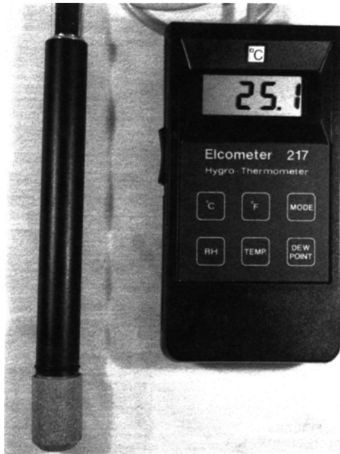
Figure 3. A digital hygrothermometer gives instant readout of air temperature, relative humidity, and dewpoint.
