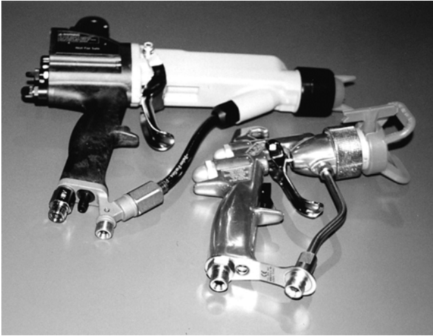
Figure 2. Air-assisted airless guns. Note tip guard, trigger lock, and reversible (switch) tip on bottom gun.
