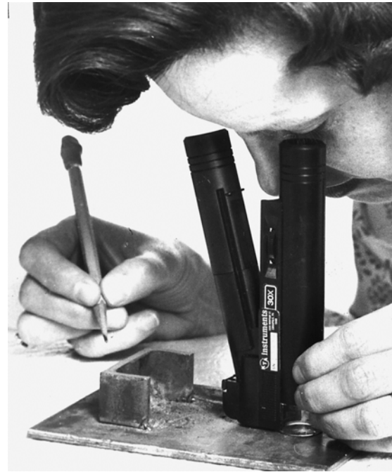
Figure 31. Pocket-sized 30X microscope with integral light source.
