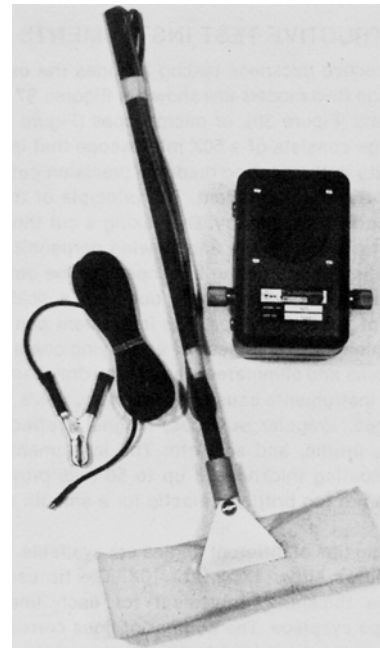
Figure 34. Tinker-Razor low-voltage wet sponge holiday detector used for finding pinholes and holidays in non-conductive paint films up to 20 mils thick when applied to conductive substrates.
