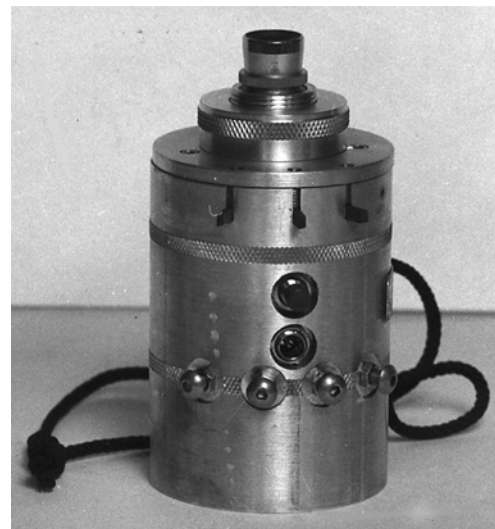
Figure 28. Tooke scratch gauge for determining dry film thickness by cutting a cross-section through the film and viewing it under magnification.
