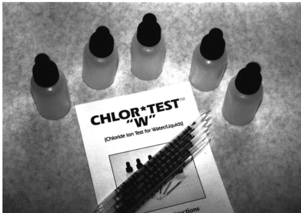
Figures 7a and b. Commercial tests kits for detecting chloride contamination on abrasive media (a) and in wash water (b).
