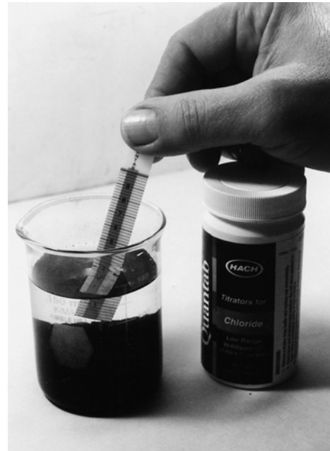
Figure 6. Testing for the presence chlorides.
