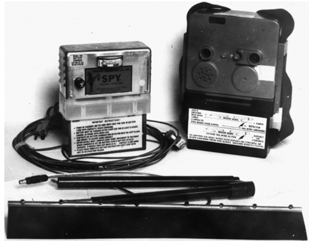
Figure 36. Spy high-voltage holiday detector for uncovering flaws in thick coating systems. Voltages are available up to 22,000 volts DC. A spark jumps from the electrode through the coating at deficient areas.
