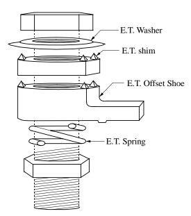
EVER TGHT DECKING ASSEMBLY Decking assembly fastener for wherever rail ties or timbers are secured to steel beams.
