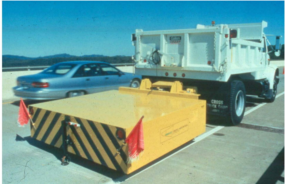
Figure 2.3.18 Shadow Vehicle with Attenuator
