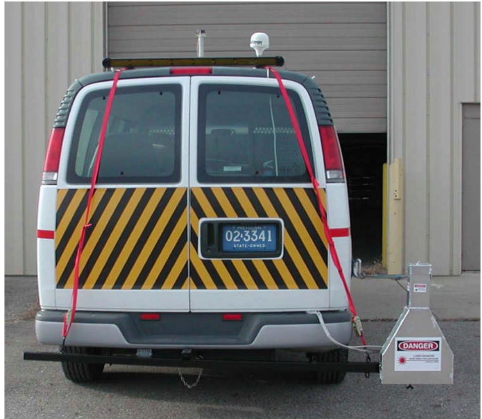
Figure 2.4.9 High Speed Underclearance Measurement System
