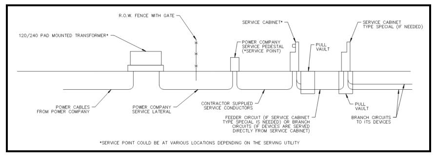
In terms of TMS design: The service conductors are the circuits from the service cabinet to the connection with the power company (service point). The branch circuit(s) are the circuits from a service cabinet or service cabinet type special to the various ITS devices. The feeder circuit is circuit between the service cabinet and service cabinet type special. Service conductors are located on the service side of the service pedestal. Figure 3-6 shows the circuit types.
