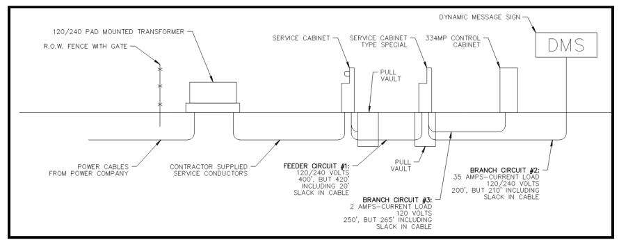
Calculating the voltage drop and size the conductors to not exceed the maximum preferred voltage drop for the feeder and branch circuits as follows:
