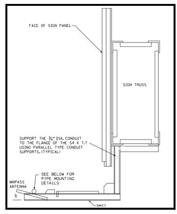
Figure 3-33: Tolling Antenna Bridge Mounting Detail
