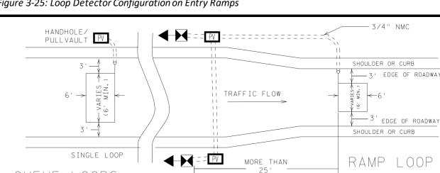
Figure 3-25: Loop Detector Configuration on Entry Ramps
