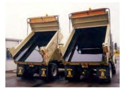
**Project Description:** These truck bedliners are designed to protect dump truck boxes from damage and allow materials to slide out more easily. The district will apply a liner to one new truck to protect it and to one damaged truck in an effort to recondition the bed.
