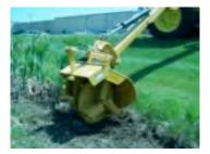
**Project Description:** This attachment has a rotary blade that is often used to clear vegetation from roadside ditches during warmer months. The district will evaluate the tool's effectiveness during the winter, using it to cut through compacted snow and ice that have accumulated in ditches. The ditching wheel attaches to a Tiger boom mower owned by the district.
