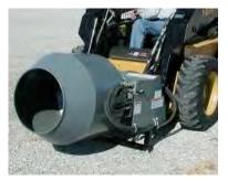
**Project Description:** This cement mixer attaches to a skid-steer loader, allowing crews to mix and pour cement on-site for maintenance and repairs such as grouting culverts. The mixer has a 5-cubic-foot capacity and is powered by the hydraulic system on the skid-steer loader. It attaches to all skid-steer loaders that are compatible with the quick-attach system.
