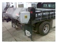
**Project Description:** This heated truck bed insert uses the truck's engine coolant to heat asphalt patching mix to a workable temperature within half an hour year-round and keep it pliable throughout the day. The system's hydraulic shoveling platform lowers materials from the bed of the truck to a comfortable shoveling height. The system allows leftover hot mix from the previous workday to be reheated to a workable temperature, eliminating the need to chip out hardened mix each morning.
