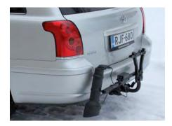
**Project Description:** This mobile road condition sensor is designed to detect the road condition and friction level (how slippery the road is) using an infrared light transmitter and a receiver. As the vehicle travels down the road, this information is then sent to a cell phone mounted on the vehicle's dash. The sensor provides continuous information to the operator on real-time road conditions.
