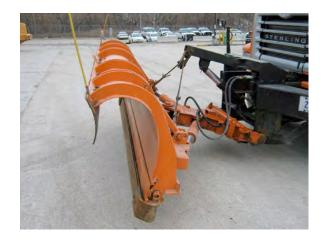
**Project Description:** The district's snowplow operators tested two Winter Equipment cutting edges to determine whether the blades have a longer wear life than the blades now in use.
