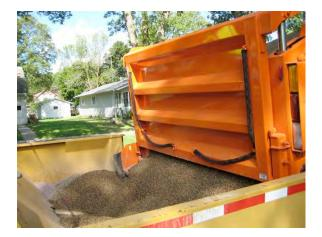
**Project Description:** The material control gate replaces a conventional tailgate and is used for dispensing hot mix and shouldering material. This multifunction tailgate was mounted on a Class 35 dump truck with an elliptical box.
