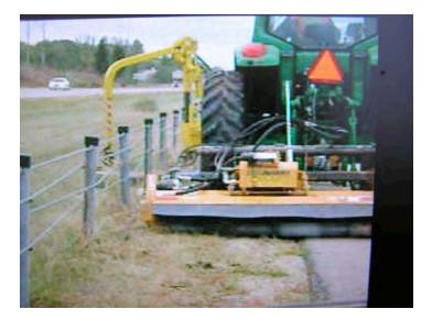
**Project Description:** A side shift mowing system allows mowing crews to mow the entire area next to median cable guardrail in one cut using a tractor mounted with the Spider guardrail mower. The two-disc mowing system can simultaneously cut from both sides and underneath an obstacle.
