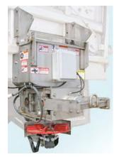
**Project Description:** Demonstrations have shown that applying salt as a slurry mixture reduces salt application rates and improves regain times. The Monroe RTS Replacement Tailgate Sander with roller mill slurry spreader can be used for this type of salt application. While the roller mill slurry spreader was developed for a live bottom V-box spreader, the spreader's manufacturer indicated that the unit can be used with the district's newer plow trucks that have elliptical boxes.
