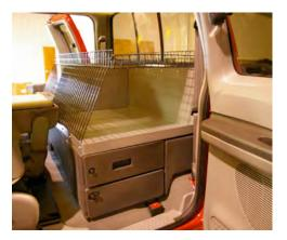
**Project Description:** The back seats of supervisors' pickups can be packed full of supplies, equipment and paperwork. These unsecured objects can be unsafe in the event of an accident and pose a security issue if valuables are in full view of potential thieves. The TruckOffice storage unit organizes paperwork, files and technical data, provides safe, secure laptop storage, and comes with an optional power inverter that can help with the use of electronics and other instruments in the field.
