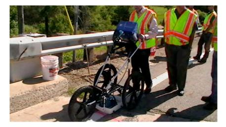
**Project Description:** Mn/DOT staff evaluate concrete bridge decks for delaminations on a regular basis using manual detection techniques, such as chain dragging and core sampling. These manual techniques are labor intensive, rely on human interpretation of acoustic feedback and may yield inaccurate results. The Ground Penetrating Radar (GPR) Bridgescan System uses an electromagnetic evaluation technique that could alleviate these problems.
