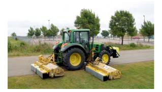
**Project Description:** In right of way maintenance, mowing is an expensive and labor-intensive operation. For many years, roadside maintenance programs have used herbicides in an effort to extend the mowing cycle. A wet cut mowing system creates efficiencies by combining the operations of a right of way mower and a chemical applicator for applying chemicals such as herbicides to stubble remaining after the mowing operation has been performed.
