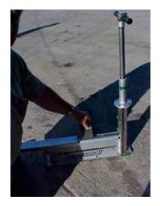
**Project Description:** Erosion blankets are used to help control soil erosion in and around roadside ditches, median ditches, slopes and culvert ends before rip-rap is placed. This staple gun is used to secure erosion blankets using 6-inch staples.
