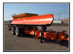
**Project Description:** The tow plow, a snowplow that can clear two lanes of traffic at once, has proved itself to be roadworthy, versatile and operator-friendly. The second generation of the tow plow includes an option for a granular box that is fitted on the frame of the tow plow that can be used in addition to an anti-ice spray bar for liquid application.
