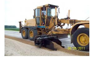
**Project Description:** The district built a wedger to attach to its motor grader to provide greater flexibility in repairing shoulders. Mounting the wedger on the blade of the motor grader allows the blade to slide left and right to do the shouldering work that is typically performed by a shouldering machine. The grader stays on the mainline pavement while the wedger smoothes the shoulder.
