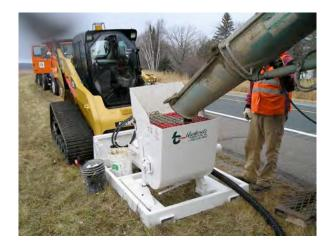
**Project Description:** The Blastcrete Model D3522 concrete/grout pump is a peristaltic pump (a type of positive displacement pump used for pumping fluids) with reversing capabilities not found in current piston pump designs. The peristaltic pump squeezes concrete out the tube for a quick and efficient pour. Simple to operate, the pump cleans up in less than 10 minutes. With its universal quick attachment to any skid steer, the pump can be used as a mobile grouting station.
