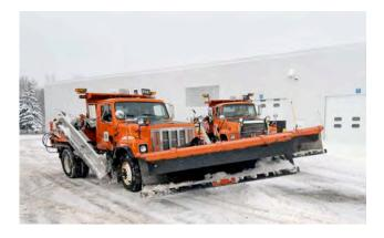
**Project Description:** Winter maintenance staff regularly wash snow and ice equipment to remove salt, but a corrosive white salt film reappears after the equipment dries. This salt film promotes the rusting process. NEUTRO-WASH neutralizes the corrosive effects of sodium chloride on radiators, condensers and other sensitive equipment parts, allowing the salt residue to be washed away.
