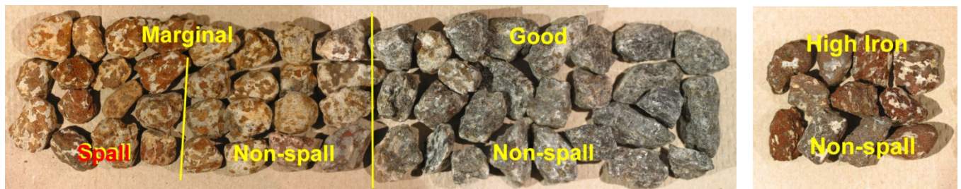
Figure 2 – Full range weathered troctolitic aggregate found in area pits from highly weathered/altere (left) to fresh (right). Also found in the pits is a metallic looking, “high iron” variety which is not considered spall (far right).
