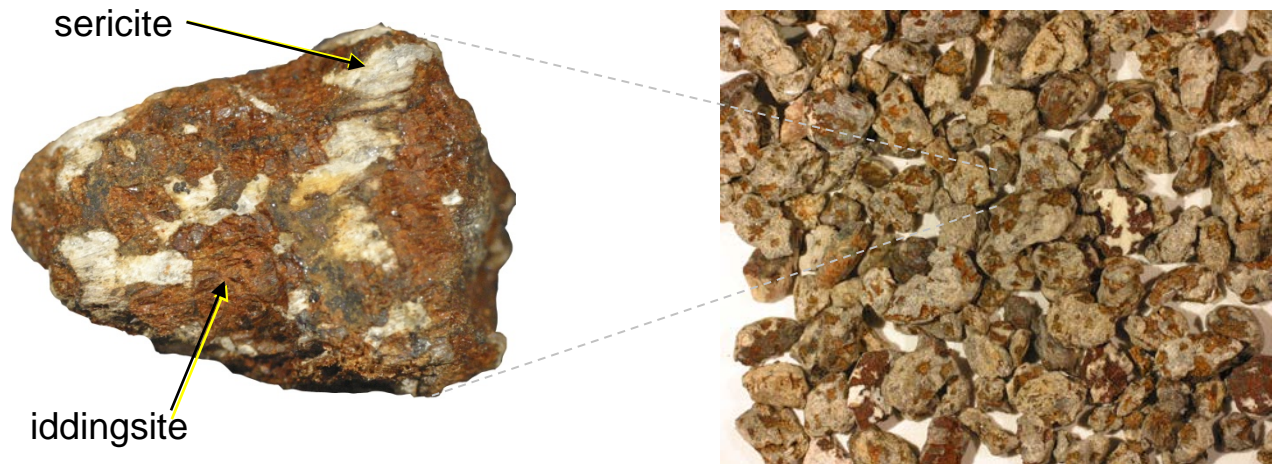
Figure 1 – 3/8-inch pile of marginal quality aggregate (right), close-up of aggregate (left)
