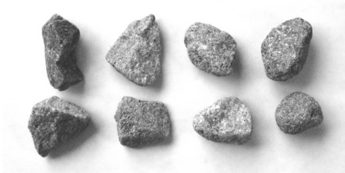
Figure 5 – Particle roundness from left to right: angular, sub-angular, sub-rounded and rounded (in natural light)
