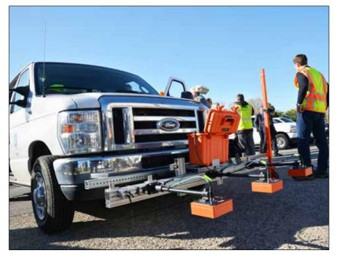
A rolling density meter (RDM) is a new non-destructive GPR technology being used in conjunction with statistical analysis model developed by MnROAD's Materials office.
